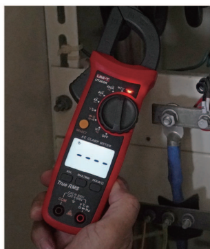
NCV multi-segment display and audio/visual alarm
