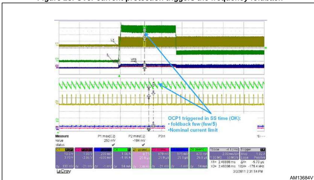
Figure 23. Over current protection triggers the frequency foldback
