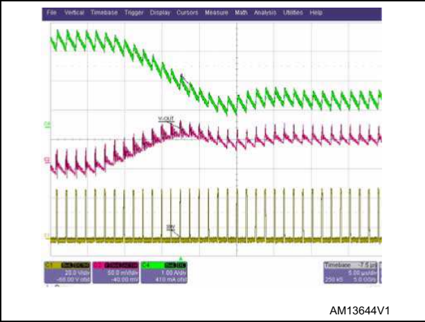
Figure 50. Zoom - 1 A to 3 A falling edge load transient ( V_{IN} 32 V)
