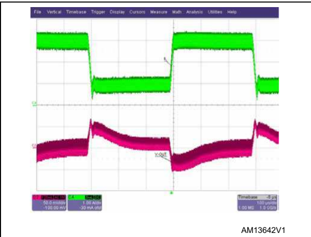
Figure 50. Zoom - 1 A to 3 A falling edge load transient ( V_{IN} 32 V)
