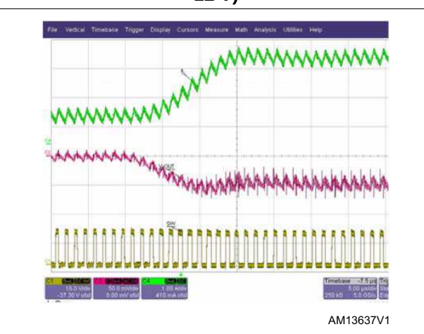
Figure 45. 1 A to 3 A falling edge load transient ( V_{IN} 24 V)
