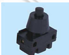
PS17A3 ON-OFF (PBS-17B) 4 A 125 VAC; 2 A 250 VAC
