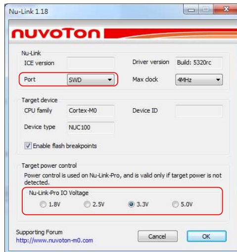
Figure 4-19 Specify the Port and Target I/O Voltage
