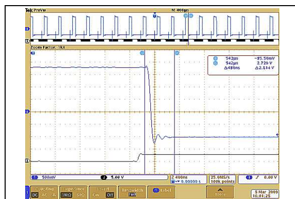
FIGURE 2-37: 10 kΩ: Write Wiper (FFh → 00h) Settling Time ( V_{DD}=2.7\text{V} ).
