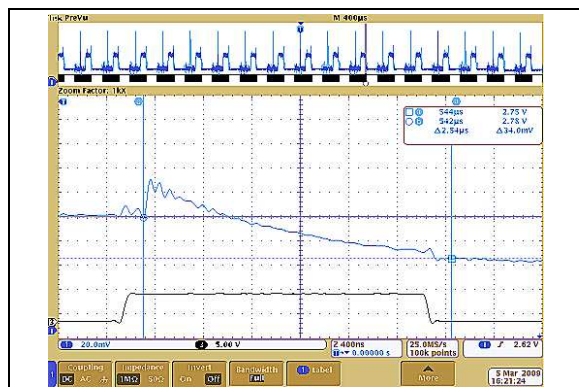
FIGURE 2-51: 50 k \Omega : Write Wiper (40h \rightarrow 3Fh) Settling Time ( V_{DD}=5.5\text{V} ).
