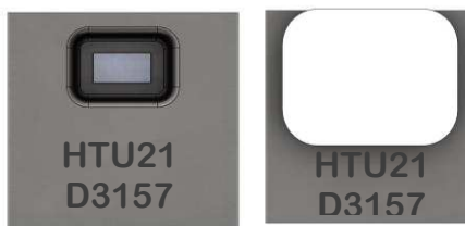
Laser marking on HTU21D(F) sensor
