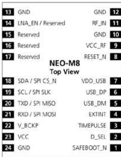
Figure 2: Pin Assignment
