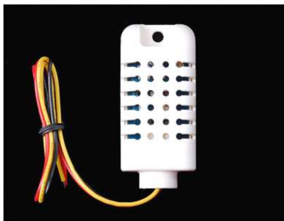
AM2302/DHT22 with big case and wires
